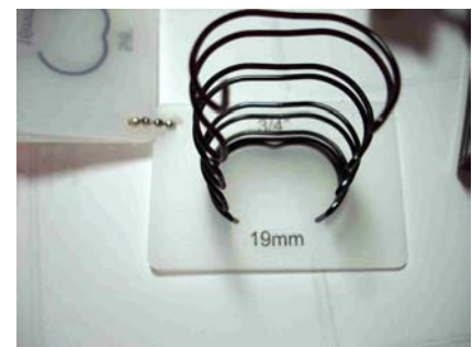
Sizing stray wire with a wire guide
