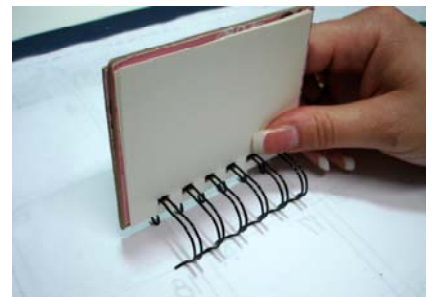
Like a bug on its feet. Narrower wire side (in back) toward the Zutter logo when pressing the wires shut.
